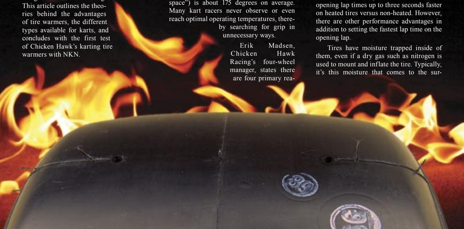
face when the tire is semi-heated, around the third or fourth lap depending on track length. Heating a tire and wheel through to the tire's carcass will bring a significant amount of this moisture to the surface (and out) and be expelled before it affects on-track performance.
