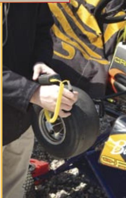
Madsen probes the baseline and sets the temperature with a digital pyrometer.
