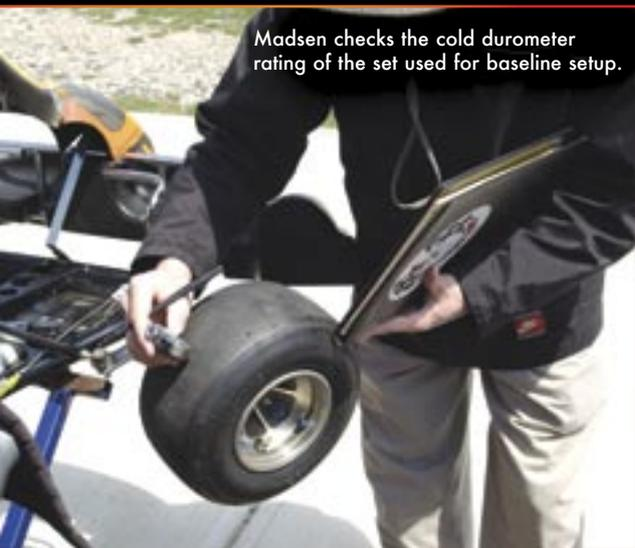
Madsen checks the cold durometer rating of the set used for baseline setup.
