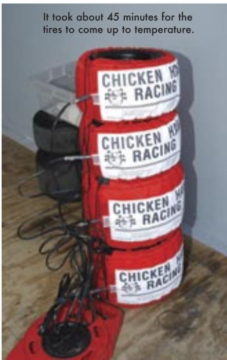
Closely tied into the performance benefits of heated tires are the tuning advantages. Tire warmers allow the tires to be set to the expected hot pressures. For racers who figure stagger into their setups, warm tires and hot pressures allow for a more accurate measurement of stagger before leaving the pits. Finally, when there is a choice between soft and hard tires, tire warmers help make that decision easier.
