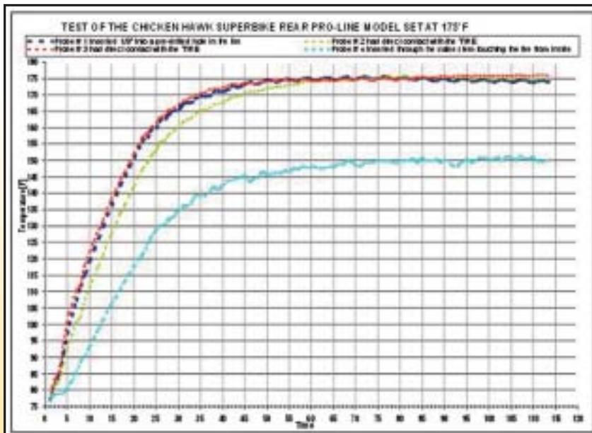
This graph shows the carcass temperature as well as the surface temperature. A thermocouple-equipped data logging system provided the inside information through the rim to the computer.
