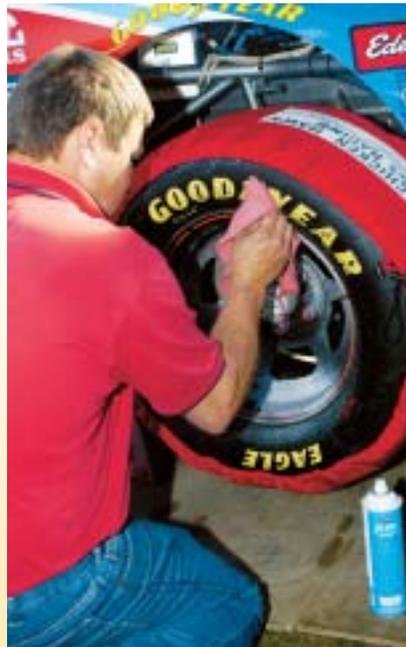
A crewmember cleans the tires already in the warmers. While the surface rubber heating is obvious, the carcass of the tire is picking up needed temperature as well.
