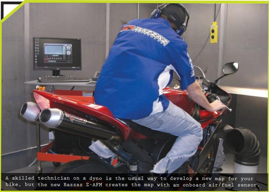
A skilled technician on a dyno is the usual way to develop a new map for your bike, but the new Bazzaz Z-AFM creates the map with an onboard air/fuel sensor.
